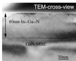
Fig3: X-Ray diffraction patterns of strained InGaN layer grown on a MOCVD-GaN template and its TEM image.
