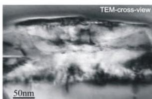
Fig 4: Complete photoluminescence spectra at different laser excitation wavelengths and TEM image of  $\text{In}_{0.6}\text{Ga}_{0.4}\text{N}$  layer undergone complete phase separation.
