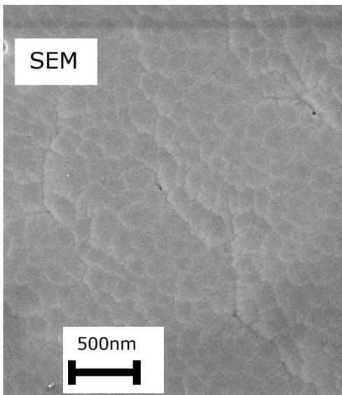
Figure 1 : Plan-view scanning electron microscope image of the p-doped GaN layer surface
