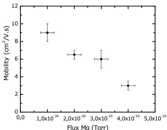
Figure 2: Hole density, resistivity and mobility of p-doped GaN layers as function of magnesium flux
