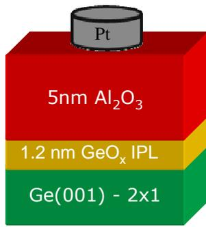
Fig. 3: Formation of a Pt/Al<sub>2</sub>O<sub>3</sub> /GeO<sub>x</sub>/Ge stack.
