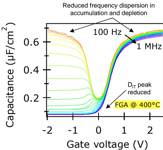
Fig. 7: C-V characteristic of Pt/9nm  $\text{Al}_2\text{O}_3/1.2\text{nm GeO}_2/n\text{-Ge}(001)$  MOS structure, exposed to FGA (10%  $\text{H}_2/90\%\text{N}_2$  for 5 minutes at 400°C).
