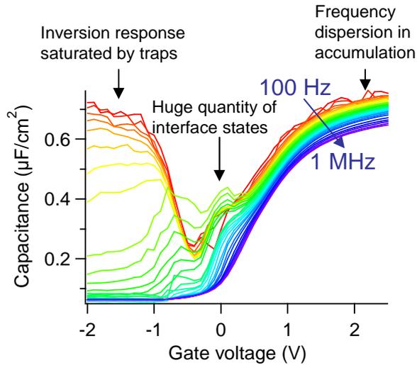
Fig. 6: C-V characteristic of as deposited Pt/9nm  $\text{Al}_2\text{O}_3/1.2\text{nm GeO}_x/n\text{-Ge}(001)$  MOS structure.
