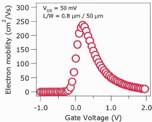
Fig. 10: Electron mobility as a function of the gate voltage for transistor structures based on Pt/Al<sub>2</sub>O<sub>3</sub>/GeO<sub>2</sub>/n-Ge
