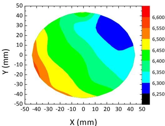
Fig. 2: Ellipsometry mapping of a 5nm  $Al_2O_3$
