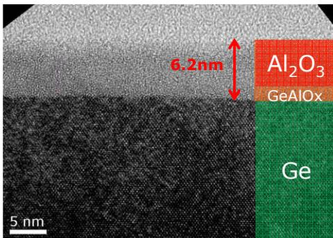
Fig. 4: TEM analysis of a 5nm Al<sub>2</sub>O<sub>3</sub> / 1.2nm GeAlO<sub>x</sub>/Ge (001) stack.
