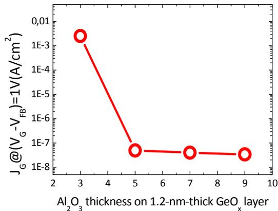
Fig. 9: Leakage current as a function of Al<sub>2</sub>O<sub>3</sub> thickness on 1.2nm thick GeO<sub>2</sub>/Ge (001).
