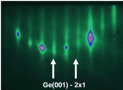
Fig. 1: RHEED pattern of a streak Ge(001) - 2x1, after deoxidation of the native oxide.
