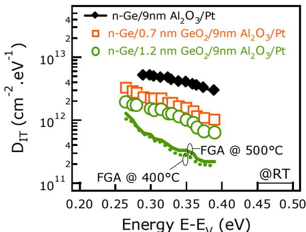
Fig. 8:  $D_{IT}$  as a function of the Energy for different MOS structures:  $\text{Pt}/\text{Al}_2\text{O}_3/n\text{-Ge}$ ,  $\text{Pt}/\text{Al}_2\text{O}_3/\text{GeO}_2/n\text{-Ge}$  with and without FGA exposition.
