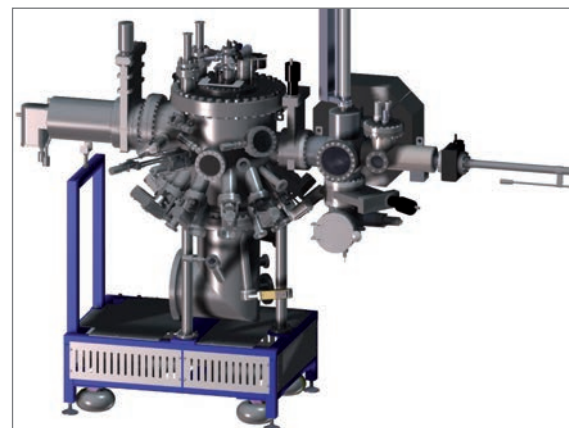
Growth chamber bottom flange with electron beam capability
