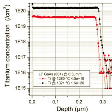
SIMS profile on low temperature GaAs(001) doped with Titanium. Titanium doping is performed at two temperatures, 1321°C and 1260°C. Deposition rates reach 2.510-2 Å/sec and 6.810-3 Å/ sec, respectively. A stable and reproducible Titanium flux profile is obtained run after run.
