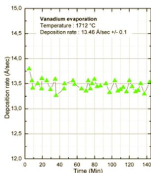
Vanadium evaporation at 1712°C shows stable flux at 13.5Å/sec.
